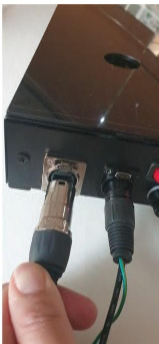
**2** Take out all 3 components of the power source: power cable, power adapter, and power connector. Connect all 3 accordingly and connect the “Power Connector” end directly to the sensor as shown below. Turn on red switch.
